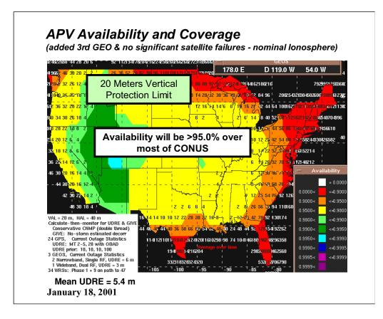
This chart shows the coverage at a **Vertical Protection Limit of 20 meters** for CONUS when the APV is attained. The yellow of the central US indicates availability above 95.0%. Most of the mountain west, in two shades of green and blue, exceeds 98.0%. Note the main reason for increased availability in the western mountains is the addition of the third GEO.
