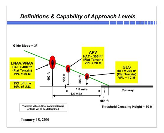
It is important to understand the definitions of the initial operational capability, called LNAV/VNAV. This first phase of deployment will provide a Vertical Protection Limit (VPL) of 50 meters or better, more than 95% of the time over at least 50% of the conterminous US (CONUS). Current analysis and expectations for this phase are shown on the next chart. This analysis shows an initial capability with availability of 95% to 99% over most of the CONUS.
