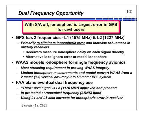
GPS was originally designed with two frequencies to primarily eliminate the effect of the ionosphere. The L1 signal has two components, a C/A code and a P(Y) code, the L2 signal currently carries only the P(Y) code. The P(Y) code is encrypted for military users, and most civilian use is restricted to the L1 C/A code signal.
