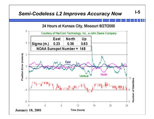
The purpose of this and the following plot is to show that *use of L2 today* is practical and leads to quite good vertical and horizontal accuracy over North America, with a reference station network much smaller than that of WAAS.
