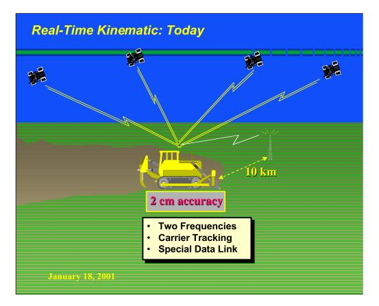
Using special differential techniques, the sophisticated civil GPS user can attain accuracies of 2 cm or better over a range of 10 kilometers to a calibrating reference station. To do this the civil user must use 2 frequencies and a special data link.
