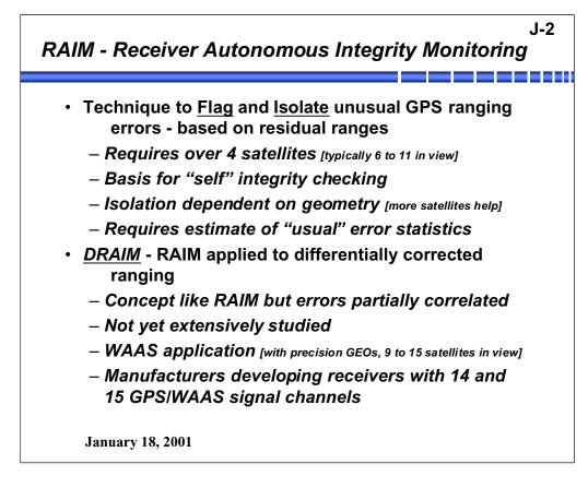
The concept of RAIM, or Receiver Autonomous Integrity Monitoring, has been studied for many years. Briefly it is a technique that uses an excess of measurements to check whether one or more are anomalous, and discard the anomalous ones from the solution. Since GPS requires four satellites to navigate, all ranging measurements over four (the "excess") allow some RAIM determination to be made.
