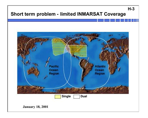
The area of dual coverage from the current INMARSAT GEOs is limited to a small portion of the service volume--just a slice of the western portions of CONUS. Should either GEO fail--either the WAAS navigation payload or the full satellite itself, the service volume would be cut nearly in half. The INMARSAT GEO covering the Atlantic Ocean Region is the the most critical for coverage in CONUS.
