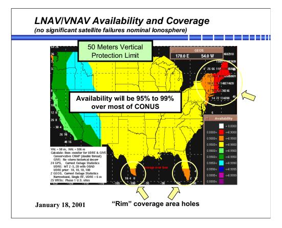
The IRB requested a careful simulation of WAAS availability over the CONUS and Alaska and Hawaii. This availability was evaluated for different system level accuracies. The results for the initial commissioning of LNAV/VNAV of the system under nominal conditions over CONUS are shown here. The GEO constellation has only two satellites, and **both are assumed to be working.** The additional assumptions for this particular simulation are shown in this small box in the lower left corner.
