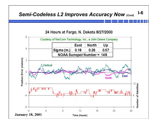
These StarFire data did not have a PDOP problem, as in the previous plot. As a result, the vertical error never exceeded two meters and seldom exceeded one meter.
