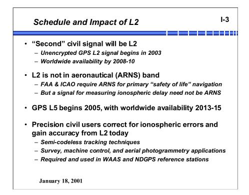
L2 and L5 will be added to the GPS constellation as current GPS satellites end their life and new ones are launched. The first L2 capable GPS launch is scheduled for 2003, with worldwide availability as shown. The first L5 capable GPS launch is scheduled for 2005, with significantly later worldwide availability. Block IIR (current replenishment GPS series) are being modified to provide L2; Block IIF (next GPS series) are being procured to include L5 as well as L2.
