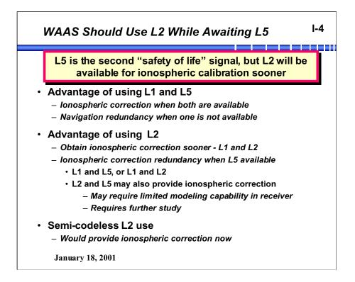
When L5 is available, aviation users will have both a redundant signal for navigation and the ability to measure the ionosphere. But they will have *access to the fully functional civil L2 signal sooner*. Since L2 is not in the ARNS band, this will only yield ionosphere calibration measurements.
