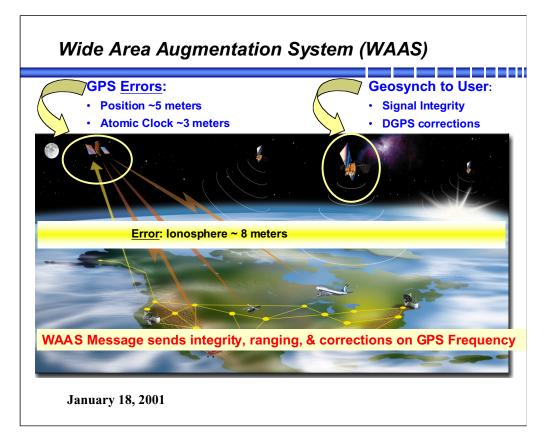
The **WAAS** concept is a **differential GPS system** designed to operate over a very large geographic region (virtually all of the US).
