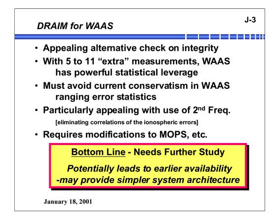
WAAS is a particularly appealing target for the RAIM (and DRAIM) techniques. *The extra ranging signals from WAAS GEOs will make it a more robust solution.* With the advent of the second frequency in a few years, the concept will be further simplified. This is because the correlations of ionospheric errors will virtually disappear.
