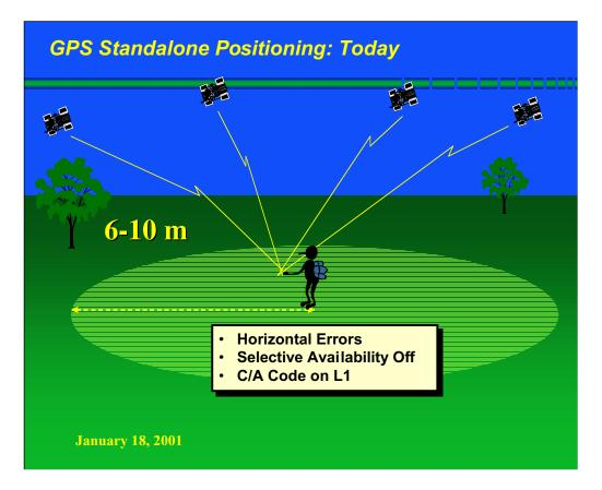
Illustrated here is typical *GPS worldwide accuracy which is 6 to 10 m horizontally*. This assumes the civil user is receiving the *L1 signal only*. Prior to discontinuing selective availability (S/A) the accuracy was typically five to eight times worse.
