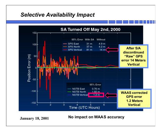
Shown is the actual positioning error during the period that S/A was turned off in May 2000. The vertical accuracy of WAAS-corrected GPS (1.2 m - one sigma) was unchanged whether S/A was turned on or not. Note this is for typical operations in the interior regions of the US.
