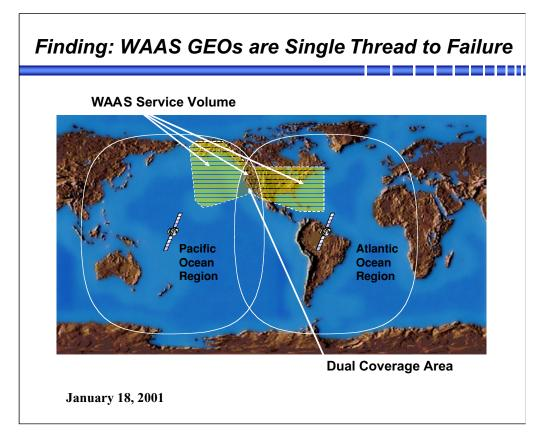
As depicted in this chart, the coverage of the two existing geosynchronous satellites (GEO) is required to cover the WAAS service volume; there is almost no overlap. One is over the Pacific Ocean and the second over the Atlantic Ocean. Clearly if either one of the satellites were to fail, coverage would be seriously reduced.
