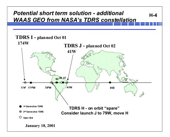
One solution briefed to the IRB by NASA would be placing a WAAS transponder on its TDRS J satellite, scheduled for launch in October 2002. This satellite is planned for 41W longitude as part of the TDRS constellation, but it could be placed in a spare slot at 79W. TDRS H is currently an on-orbit spare occupying 79W; it could be moved to 41W and operated there in lieu of J.
